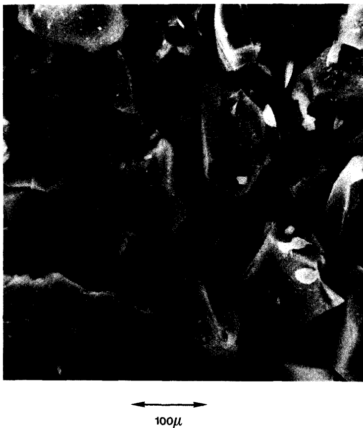
FIG. 3. Scanning electron micrograph of the \text{UO}_x\text{-SiO}_2 sample calcined at 900^\circ\text{C} . Magnification: 200\times .
